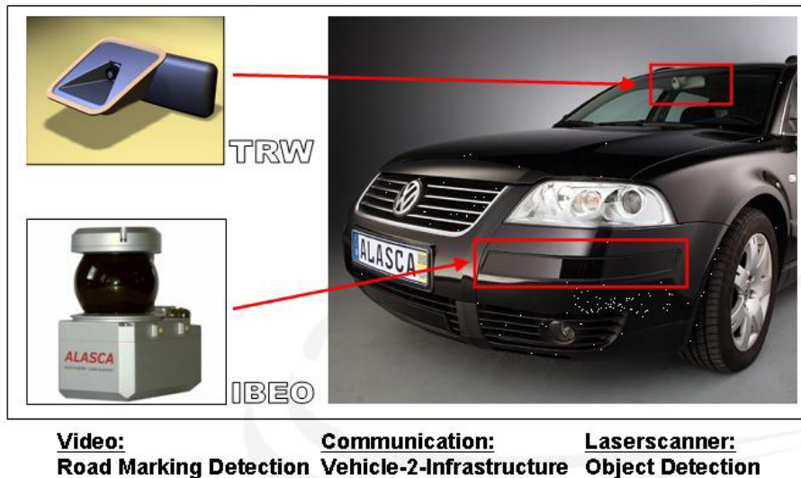
Figure 1: Bottom-Up-Approach with state of the art sensors on a VW test vehicle 1
