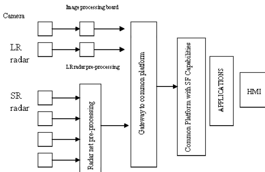
**Figure 2:** Architecture of LATERAL SAFE
