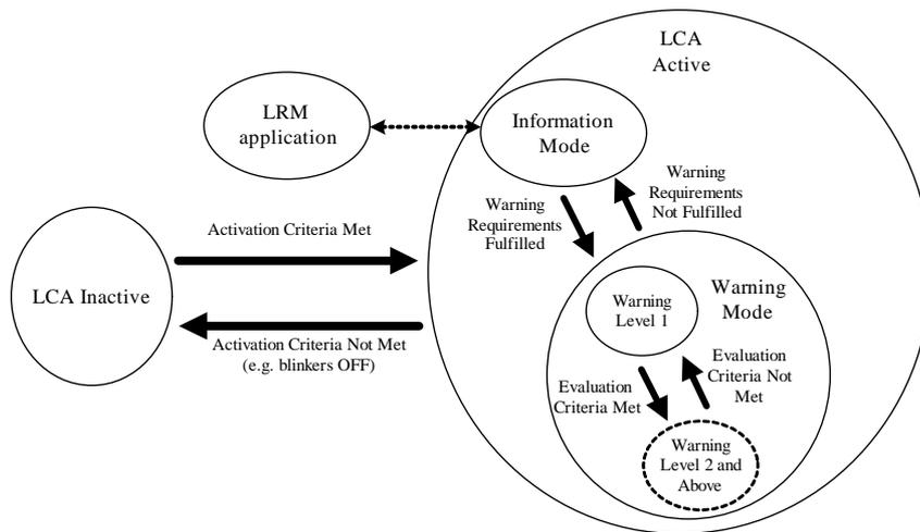
**Figure 3:** Diagram of the warning strategies in LCA application (example)
