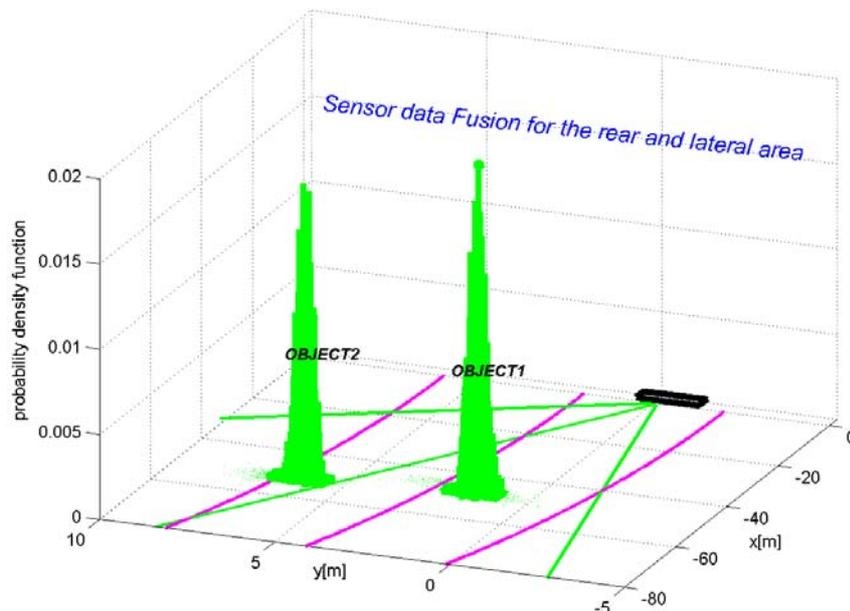
**Figure 5:** Sensor data fusion for object detection in the lateral and rear area
