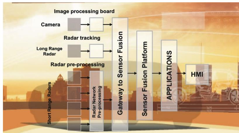
Figure 4: LATERAL SAFE basic architecture
